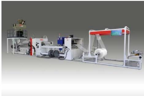
In collaboration with Meaf Holland, Rajoo presents, for the first time in Asia, a Monolayer Sheet Line with a 600 kg/hr output from a 75 mm
