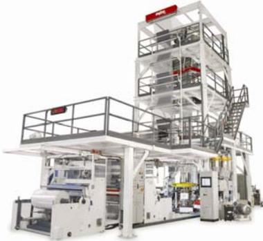
This flagship Rajoo product has made waves globally for barrier and non-barrier flexible packaging, lamination grade films, shrink films and more. To deliver high output per mm of dia (0.9-1.2 kg/hr/mm) ,
