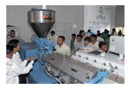
Twin Screw PVC Pipe Plant enthralled the audience when it was being operated at a capacity of 1000 kg/hr, never before seen in India. The pipe OD was 400mm and wall thickness of 16.2mm. This high output plant will now be shipped to Africa.
