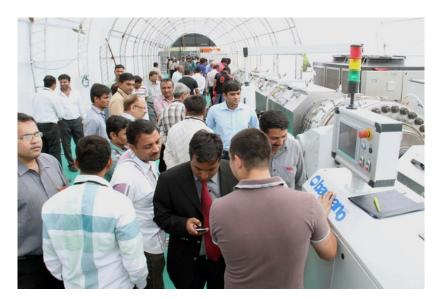
With this open-house, Rajoo marked its strong penetration into the market of Drip Irrigation pipe plants. The demonstrated line was running at 170kg/hr with a line speed of 80 MPM, 200 dripper insertions/min, with the wall thickness being 0.7mm.
