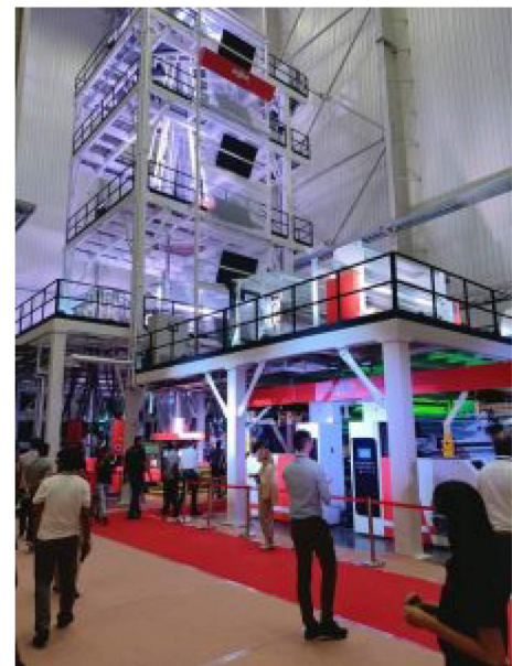
The 5-layer Proex Series blown film line in action at Balaji Multiflex in Rajkot on 5 July 2024. Photo PSA
